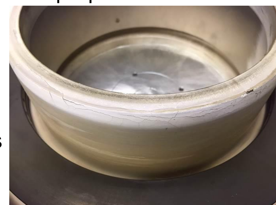
Failed HP26 BN with visible macrocracking
