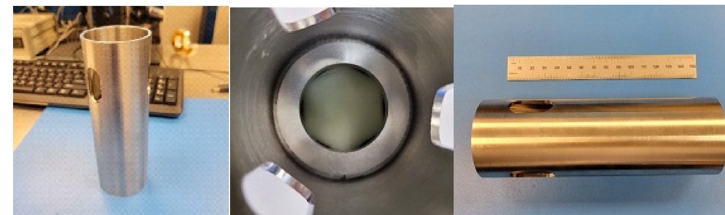
Figure 3. 3.5-cm diameter x 6.5-cm long polycapillary optic package with alignment features to mount an angular filter.
