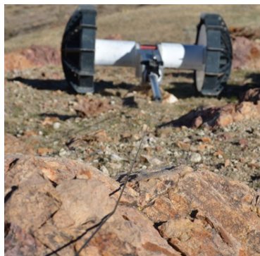
Figure 1: The Axel rover with pre-existing tether deployed out the back. Here, the tether is under tension, decoupling it from the ground, but allowing the rover to travel over challenging terrain. In Year 2, we will evaluate the use of tether deployment over both challenging and flat terrain.
