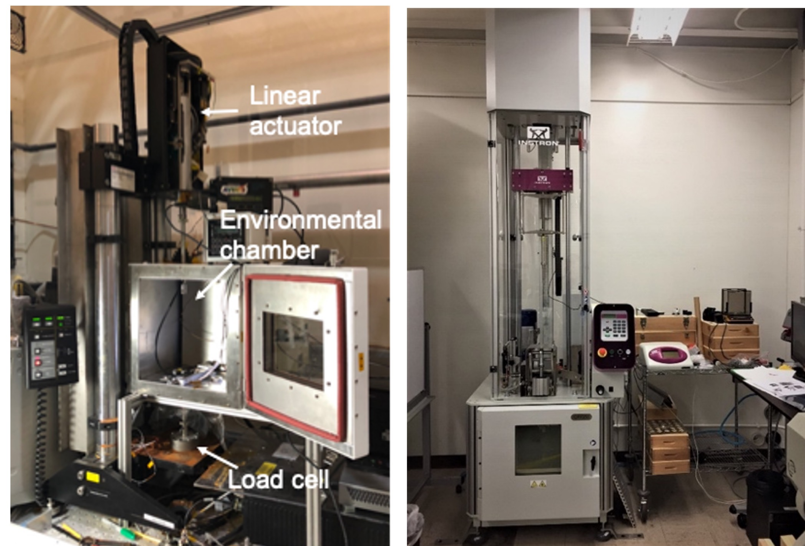
Figure 1. Left: Photograph of the cryogenic Instron press to be used for uniaxial compressive strength measurements. Right: Cryogenic Instron impact tower to be used for flexural strength and fracture toughness measurements.
