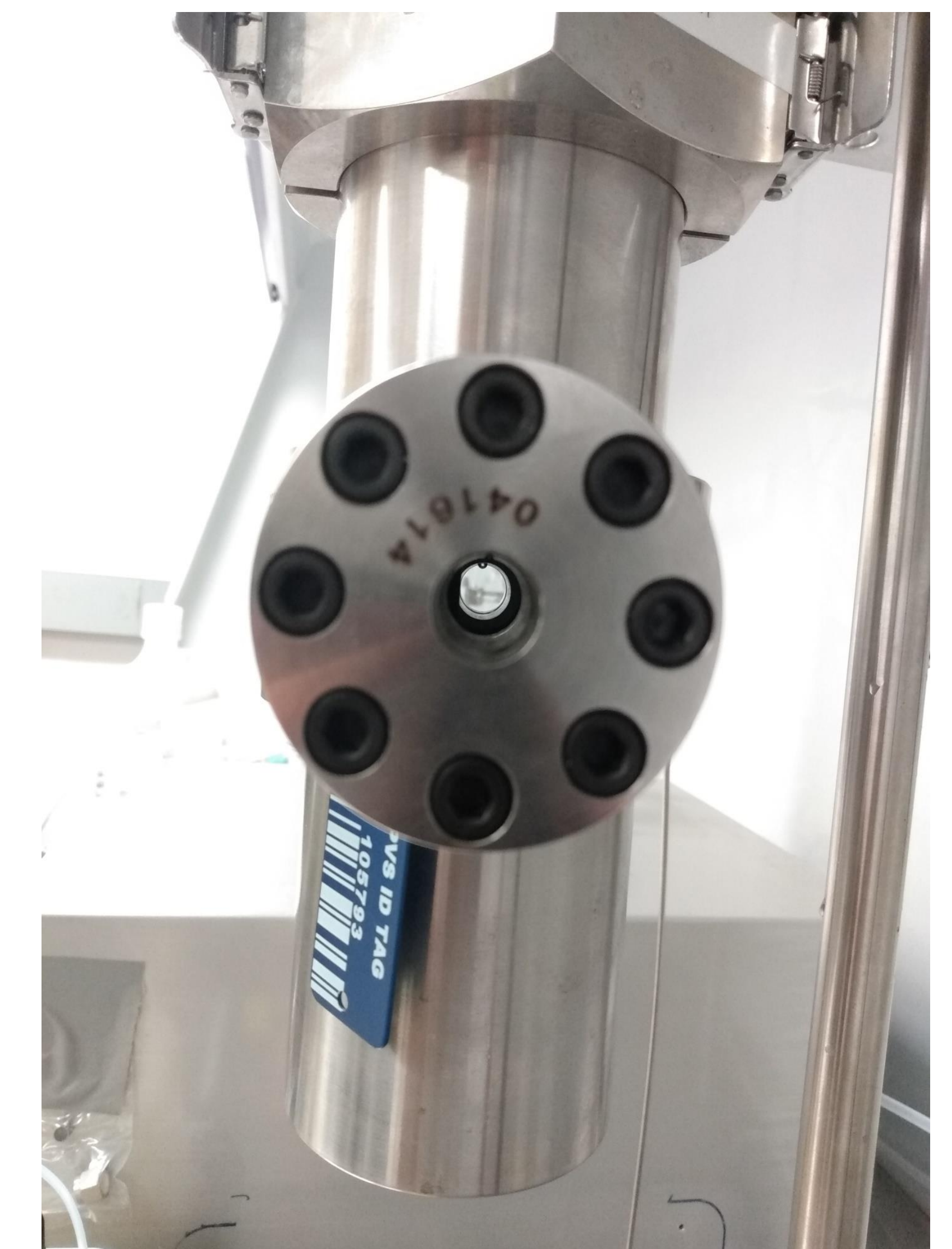
Figure 4. Photograph of pressurized reactor filled with water during pressure test at 2,650 psi.
