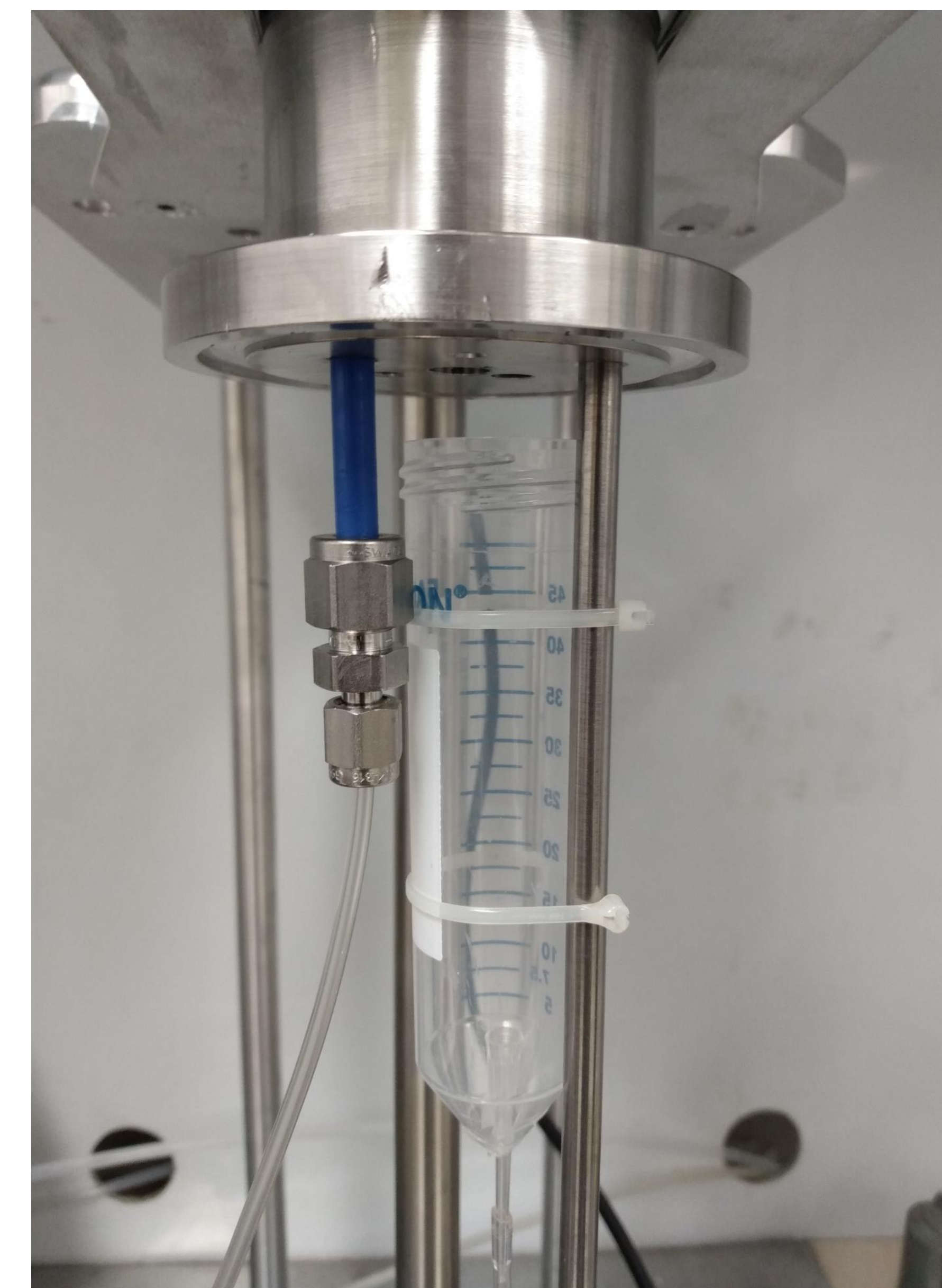
Figure 3. Image of inside of chimney growth scaffold
