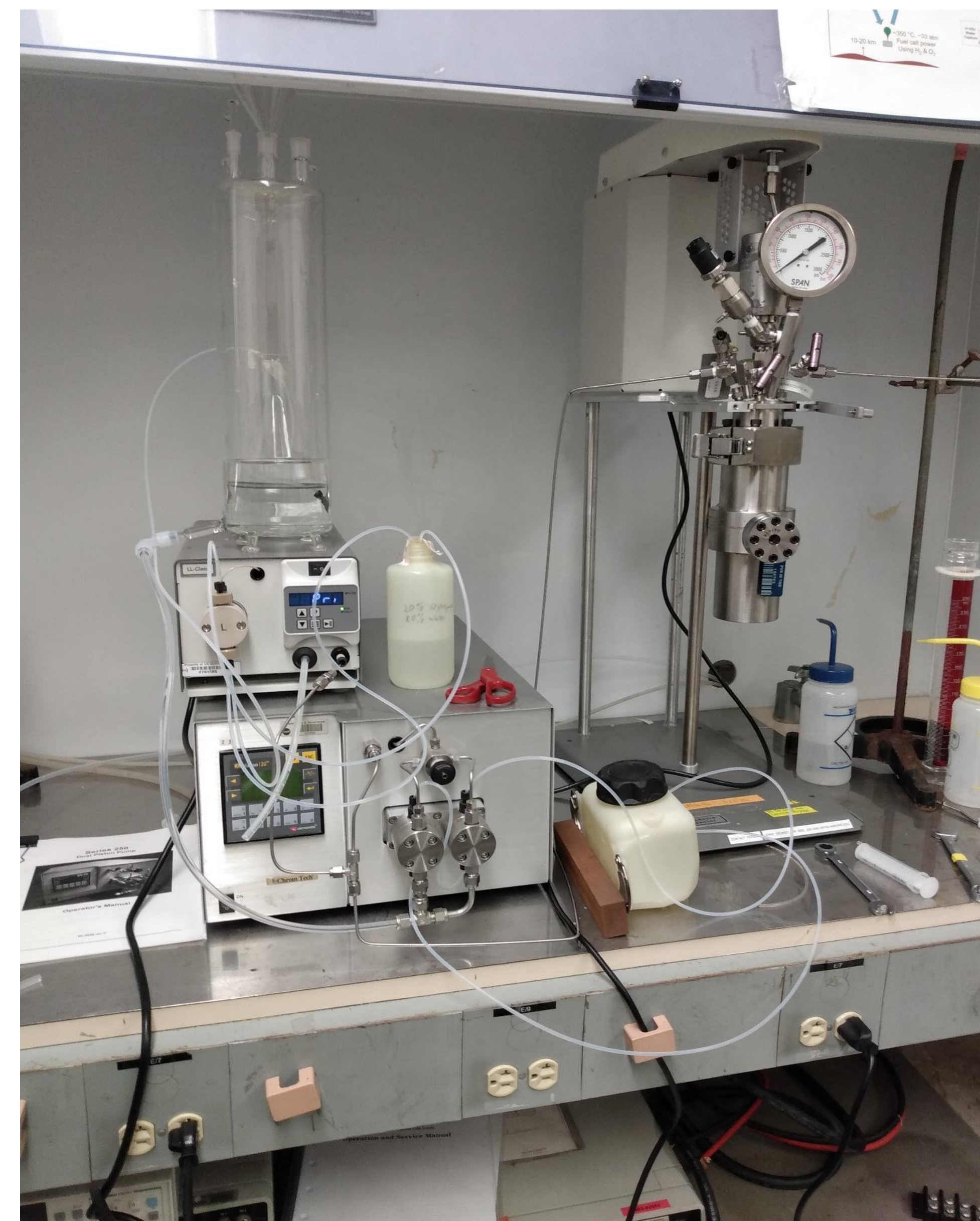
Figure 2. Photograph of reactor with windows for hydrothermal chimney growth at up to 2,650 psi and two pumps in parallel (left side of image) provide precise flow control from 0.01 to 10 mL/min.
