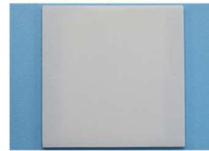
Enclosed 0.2 mm x 1 m long channel 3D printed in zirconia
