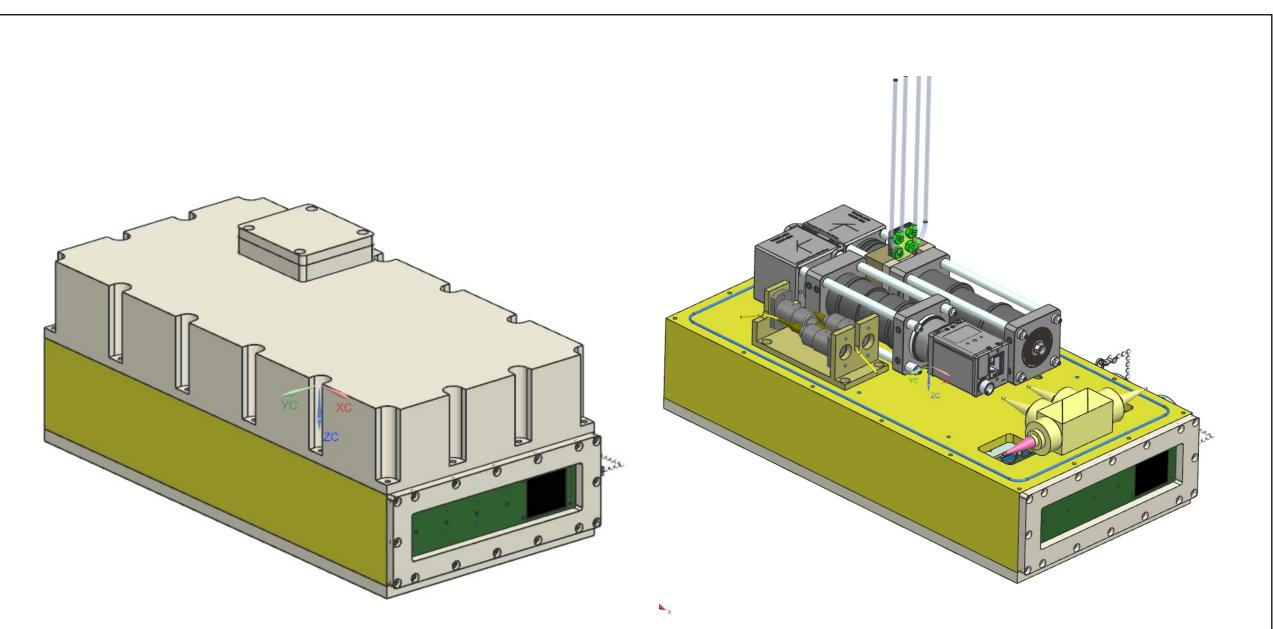
Renderings of the the digital holographic field instrument are shown above. The left image is with the cover on, the right is with the cover off. The right side shows the core of the optical instrument with holographic microscope assembly, the multiwavelength combiner, and the laser diode bracket.
