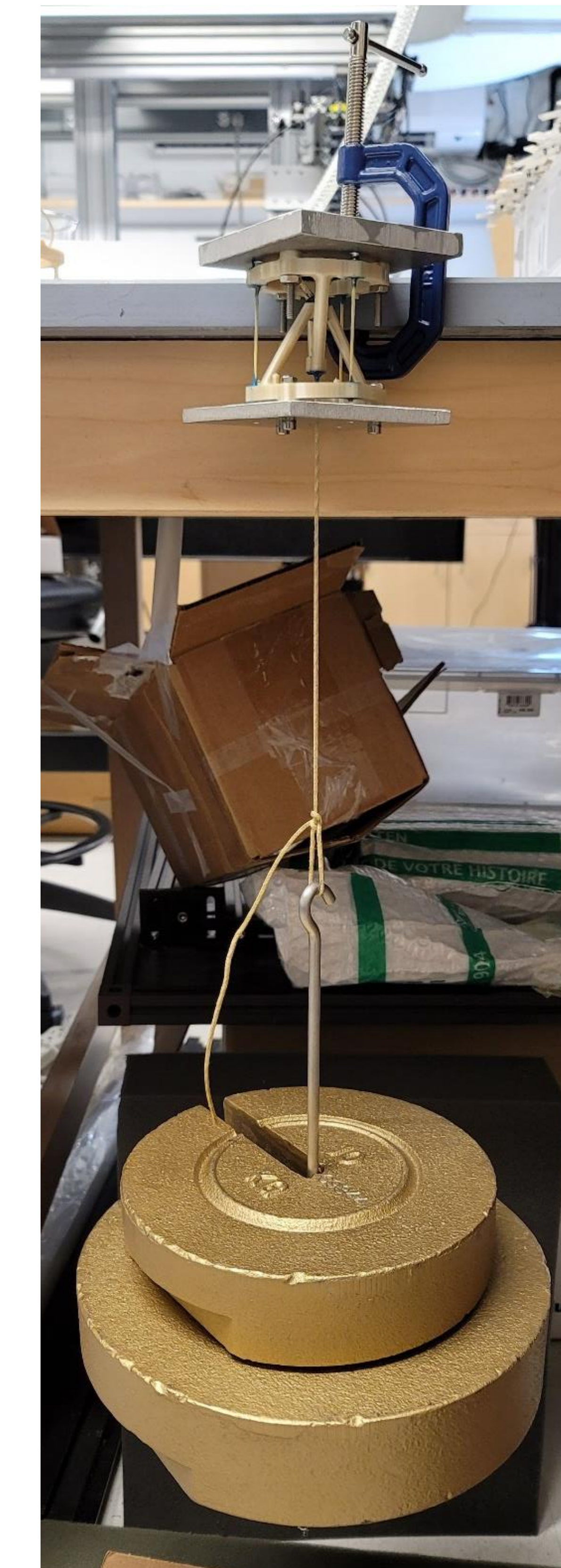
Figure 5. Final step in Tensioning one of the initial Thermal Tensegrity designs with 30kg while applying epoxy.
