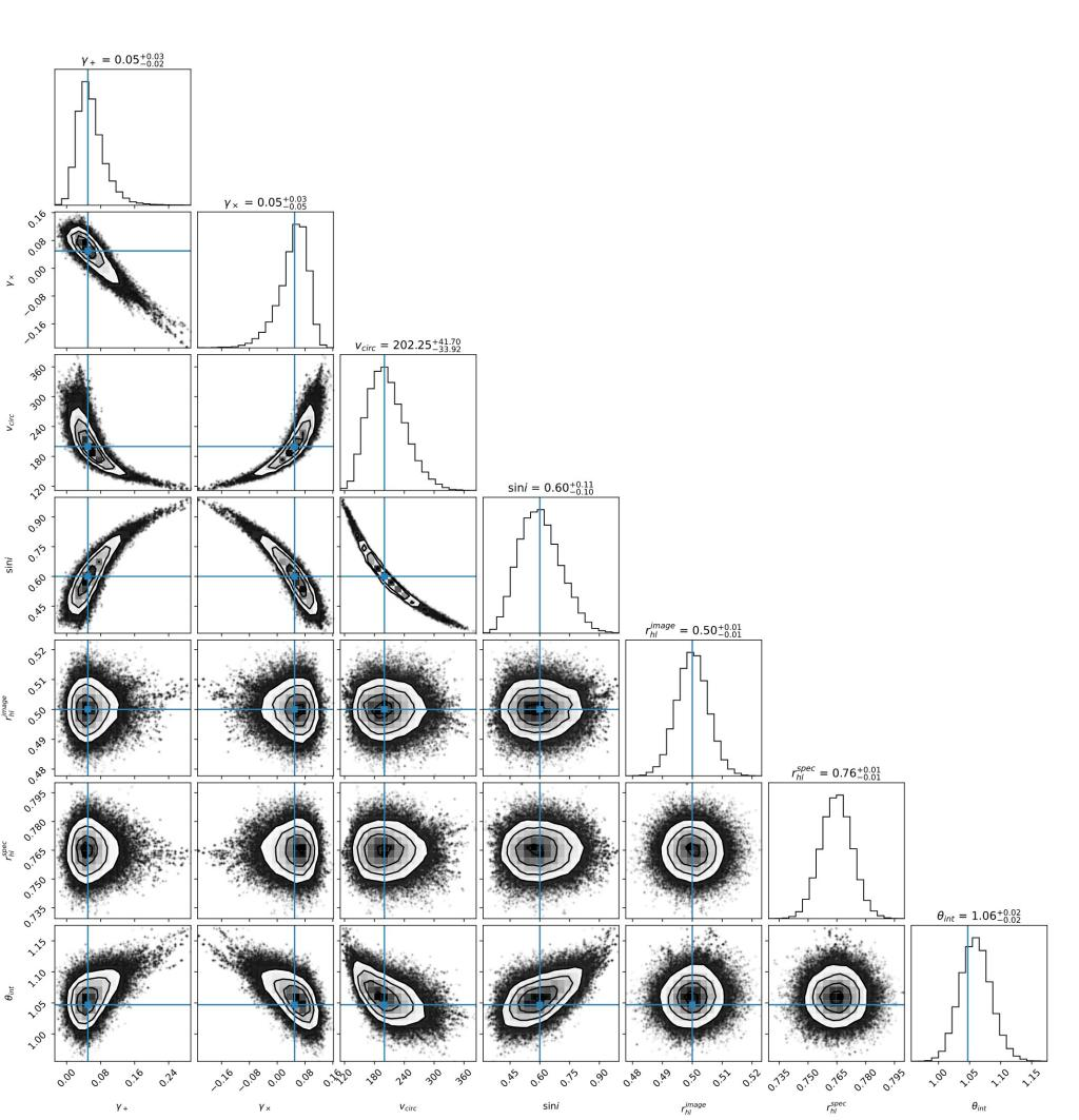
**Above:** Posterior probability distribution of parameters recovered from our simulated imaging+Keck spectra. The first two columns show the probably values of the two lensing shear parameters, given the data. The errors on the recovered values are +/- 0.025, representing an order of magnitude improvement over current techniques.
