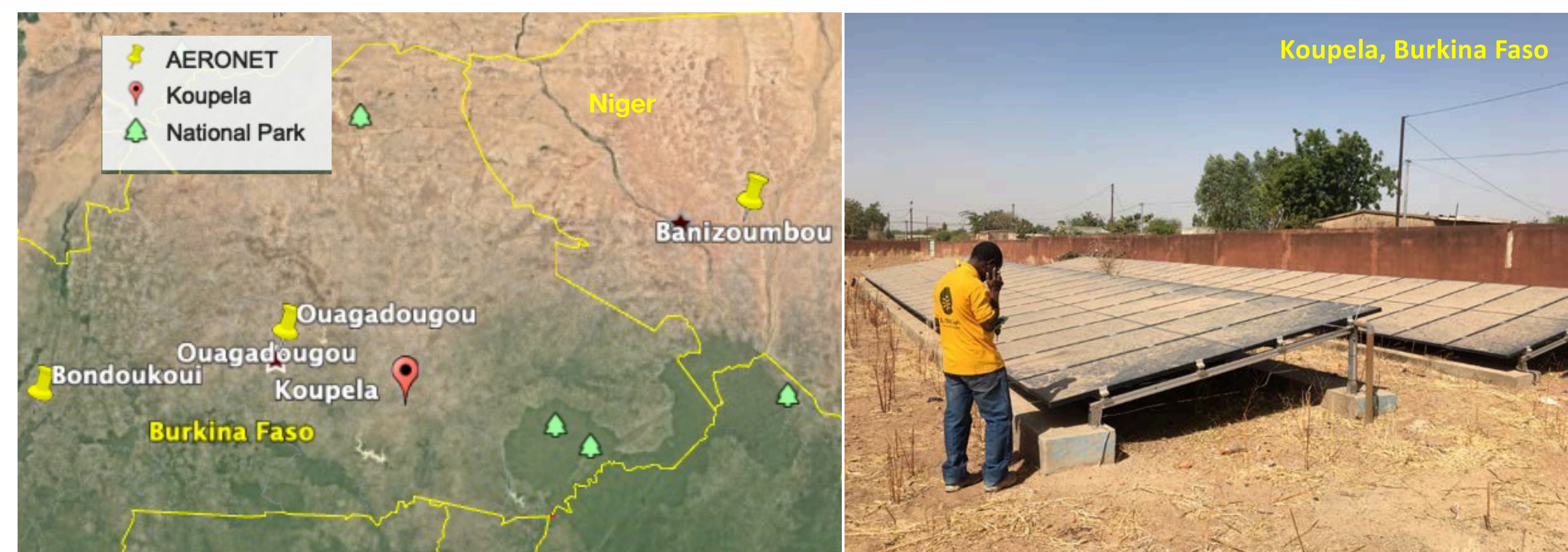
(Left panel) Location of the town of Koupele in respect to AERONET stations in Niger and Burkina Faso; (Right panel) Boureima Kabre, local leader in solar energy systems in Koupele, Burkina Faso shows a dust-covered non-operational solar system during a visit in January 2018. Credit to Stewart Isaacs, MIT graduate student.
