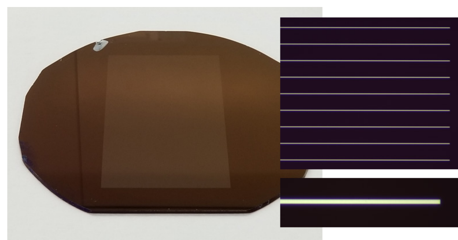
Figure 3. E-beam patterned grating of chromium lines on custom crystallographically oriented silicon wafer (6-inch dia.) to test PARVI grating fabrication process.
