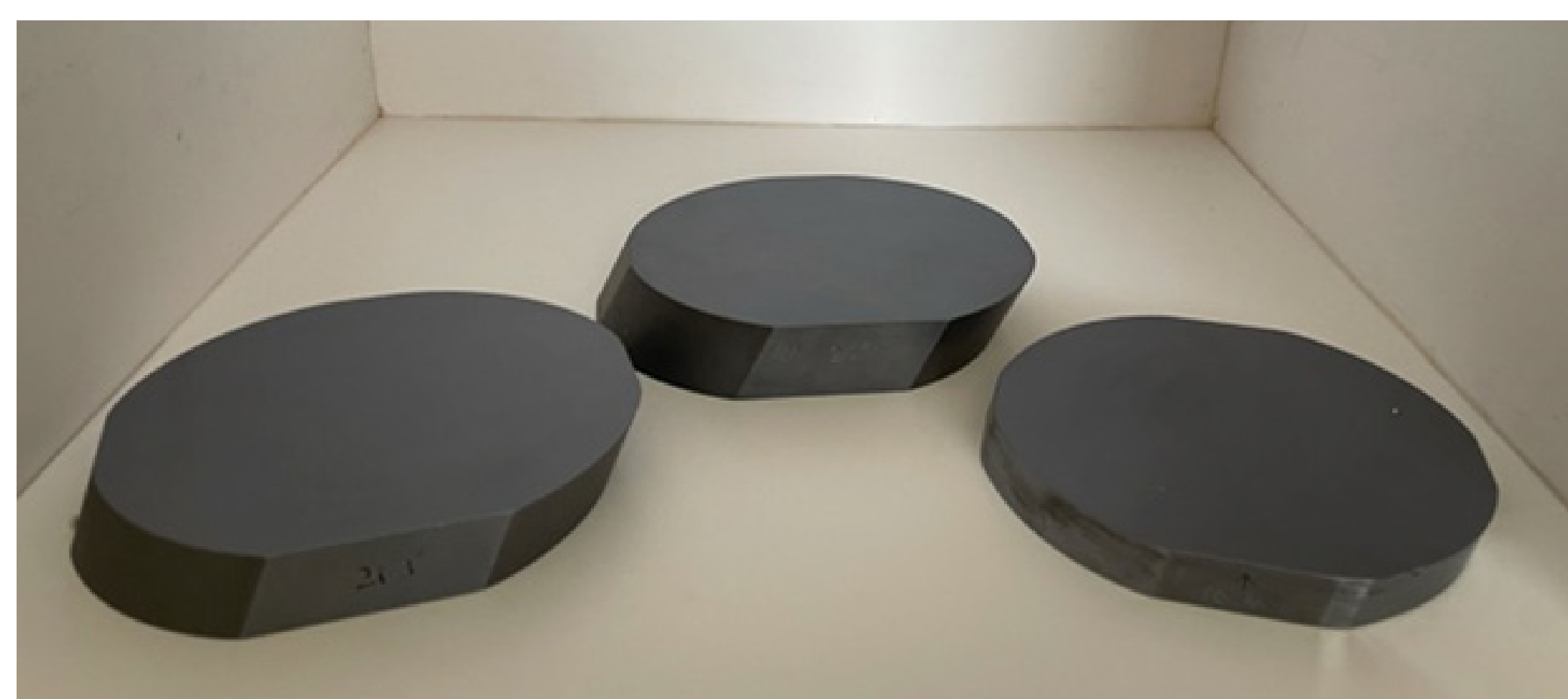
Figure 4. Grating substrates cut from custom crystallographically oriented silicon. Left to right: PARVI echelle, iLocator echelle, iLocator cross-disperser.
