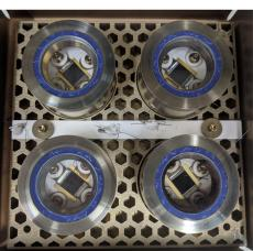
Combined-effects environmental test at JPL's Large Venus Test Chamber (LVTC) facility: temperature and pressure data acquired in-situ during test (left); Venus-Surface Solar Array test article in LVTC after exposure (right)
