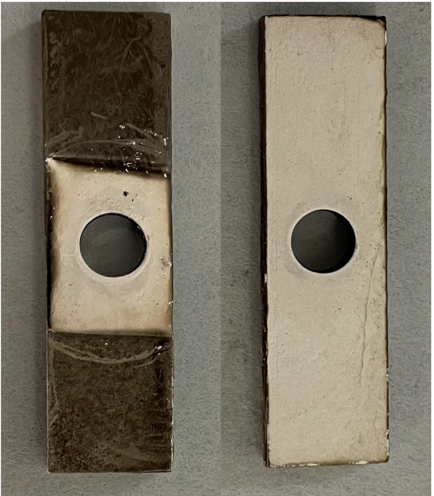
Figure 4. Figure 4: Sample A after the test sequences. Left image is the plume facing side, and the right image is the thruster facing side.
