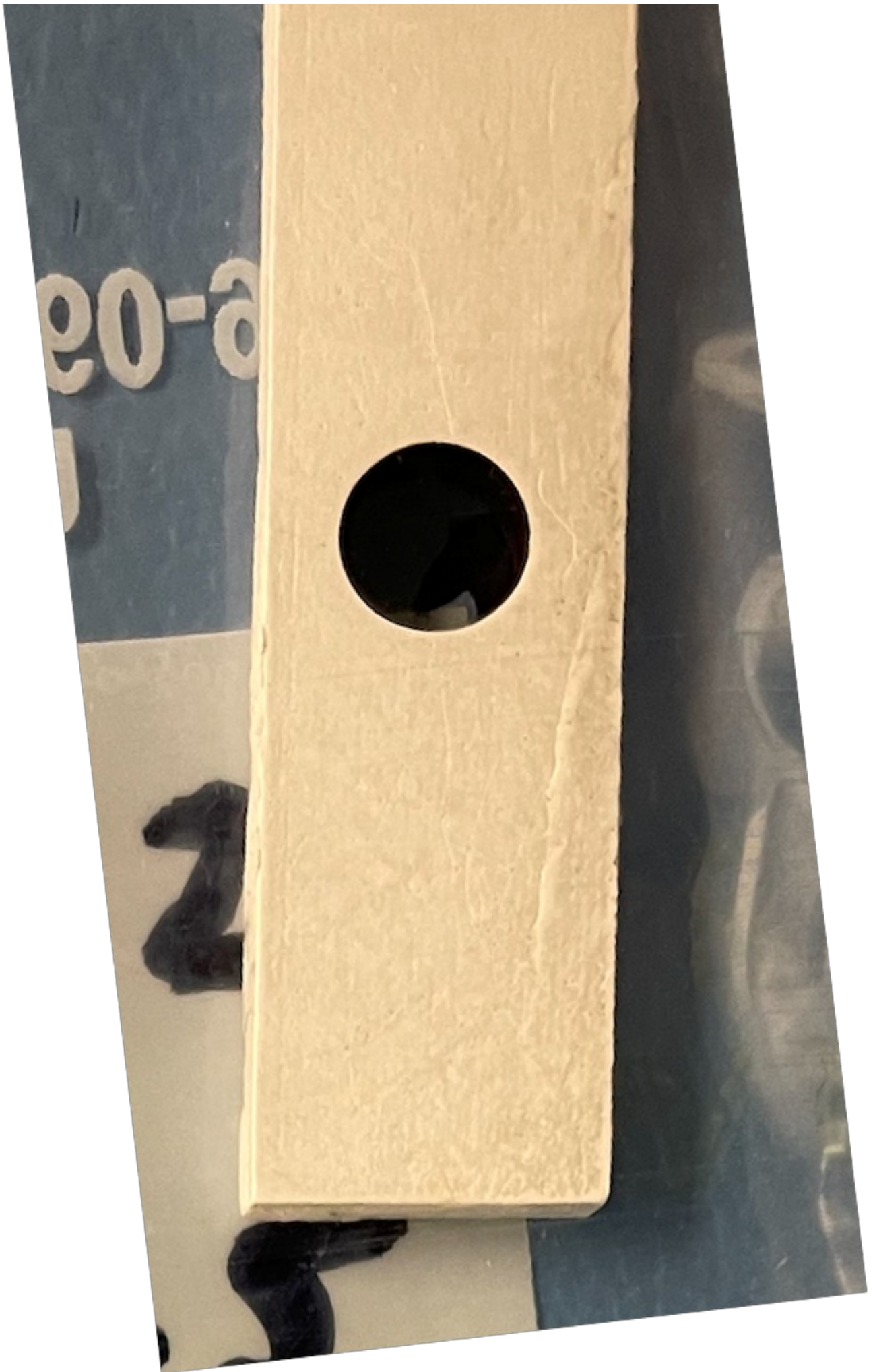
Figure 5. Figure 5: Sample A after cleaning to remove the deposited graphite layers.
