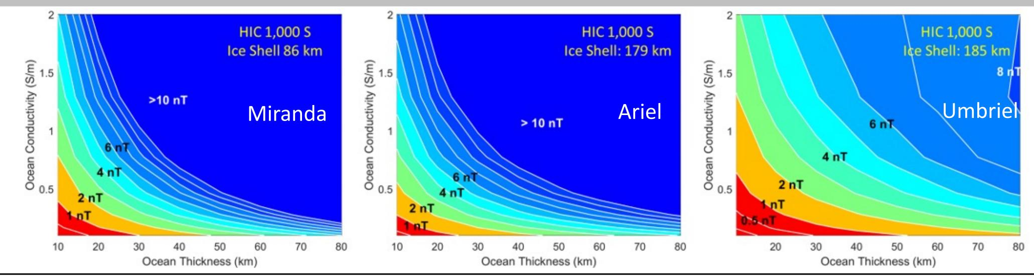
Predicted magnetic induction responses from sub-surface oceans on Miranda, Ariel, and Umbriel. These results demonstrate that detectable signatures of sub-surface oceans would be present for a range of possible ocean thicknesses and conductivities/salinities.
