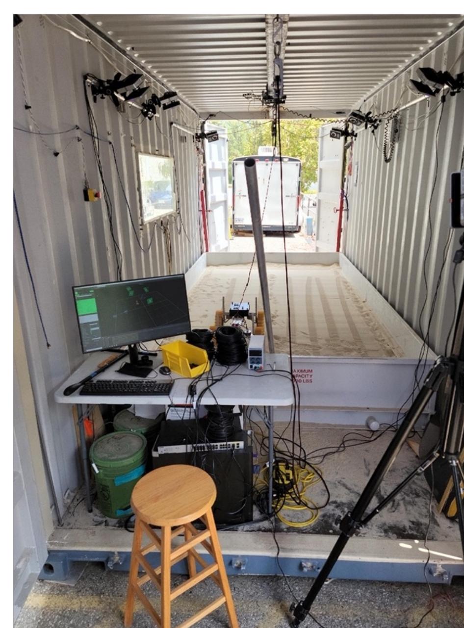
Figure 4 The experimental test facility was set up with a bed of GRC-1 lunar simulant in a ~2m wide by ~5m long by ~0.4m deep bin. The metrology system includes the Vicon motion capture system.
