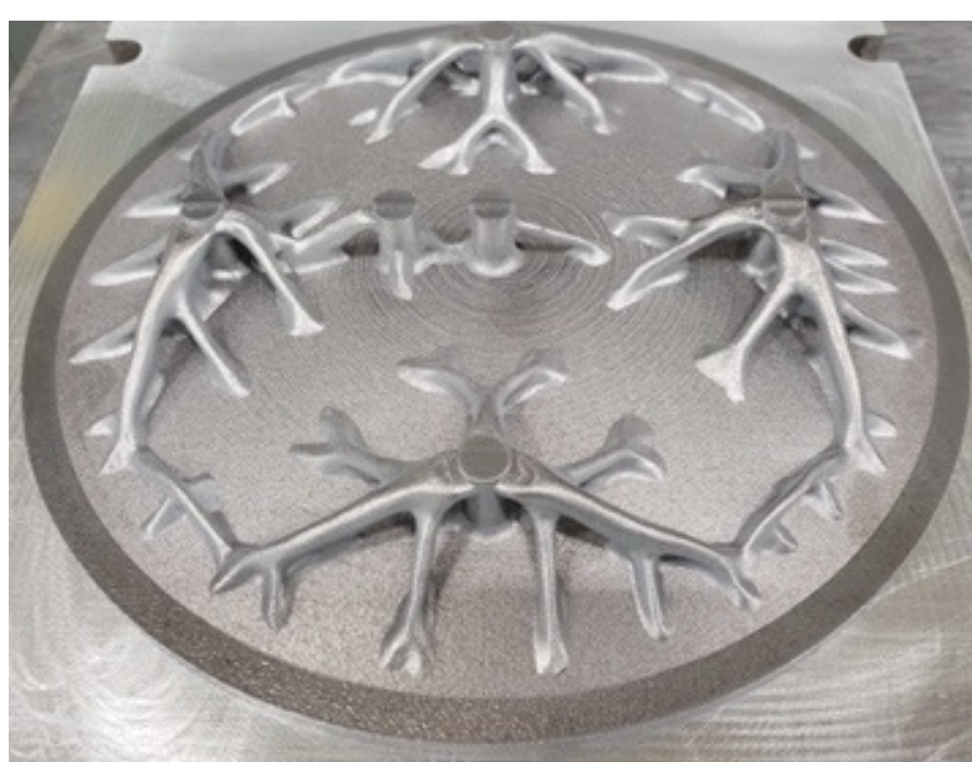
Figure 1: Front side of 8cm diameter parabolic reflector made by Additive Manufacturing with after-machining RMS of 14 \mu\text{m} .
