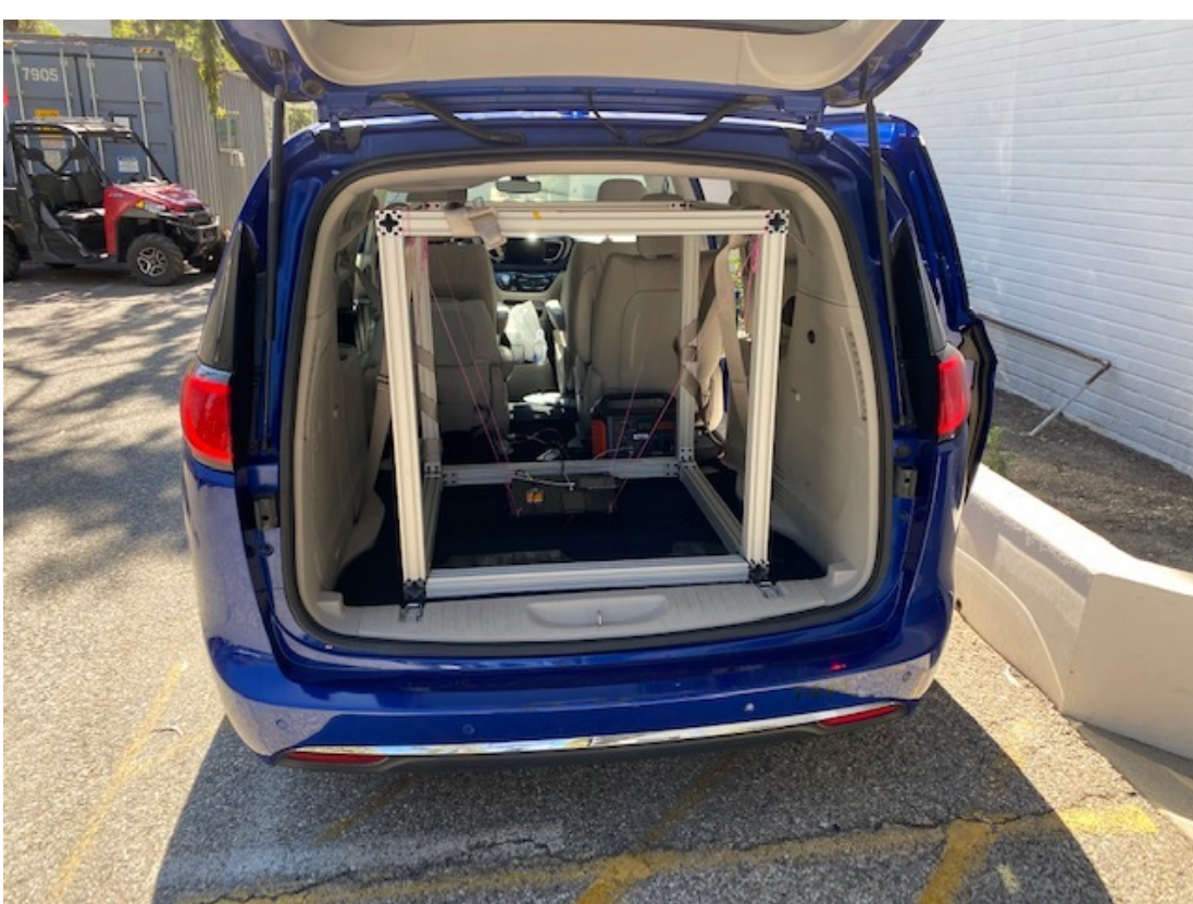
JPL Minivan utilized as a poor man's “Venus balloon simulator” by driving on the freeway.
