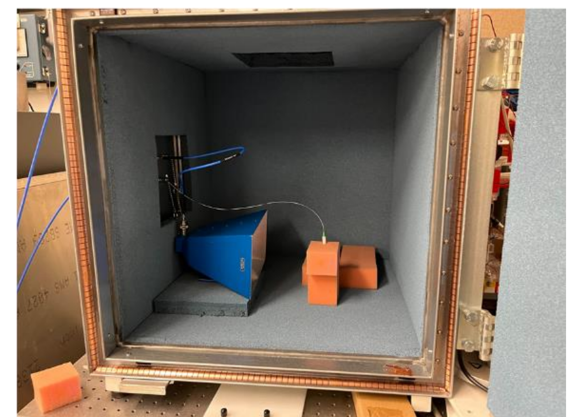
Figure 3. Experiment in an anechoic chamber, with a horn antenna driving the weak external field to the SRR to study field enhancements
