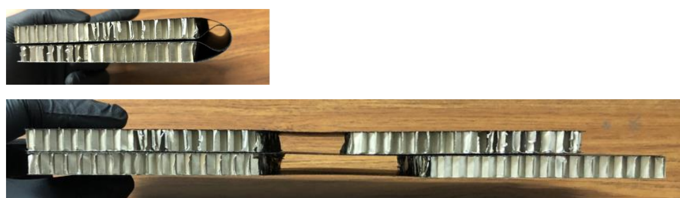
Figure 5. Proof of concept of flexure fabrication.
