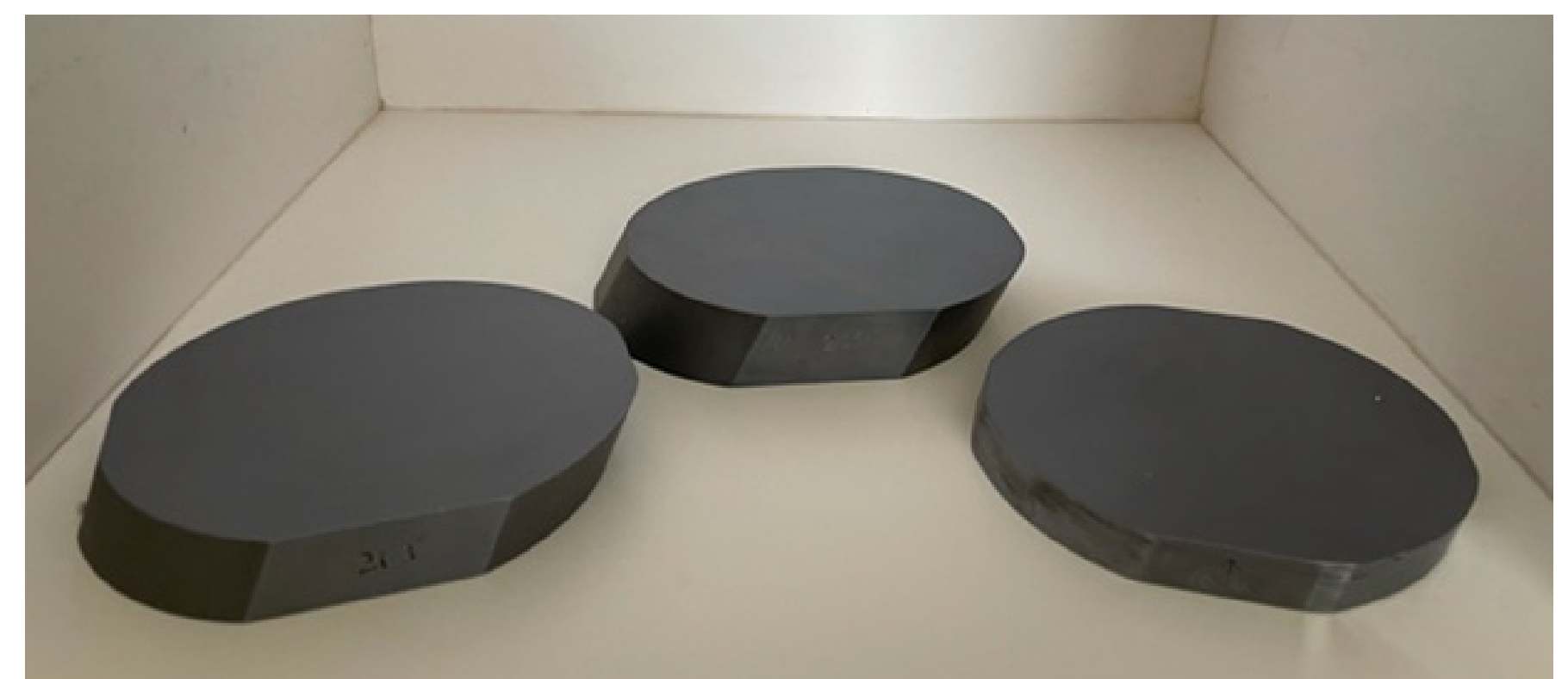
Grating substrates cut from custom crystallographically oriented silicon. Left to right: PARVI echelle, iLocator echelle, iLocator cross-disperser.
