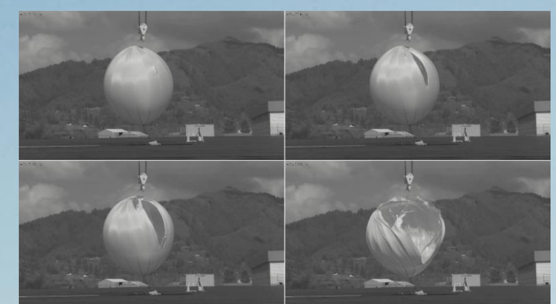
Figure 3: Stills from high-speed camera filming a pressure-to-burst test of SP balloon.
