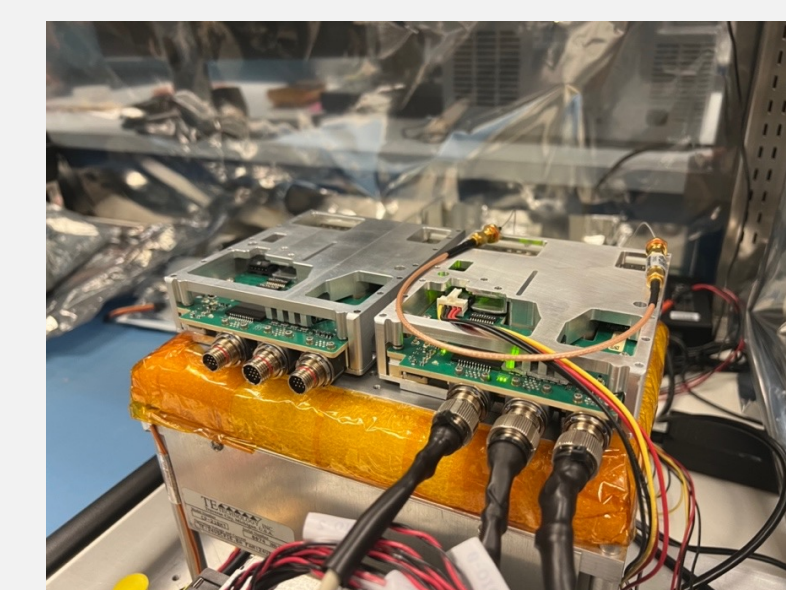
(Left) Digital test bed (COTS RF System on a Chip) for developing bistatic timing synchronization firmware. (Right) Range compressed pulse from SDRadar FPGA core.
