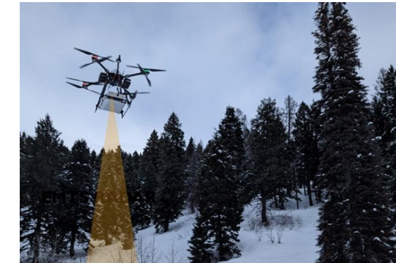
IIP-19: Ku-band MTS LP Demonstrated on a UAV snow radar (TRL 5)
