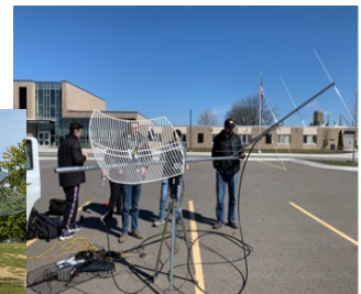
Figure 2 – A portable S-Band and VHF communication ground station.
